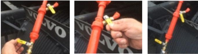
Make sure all valves on the INJECT-AIR are shut.
