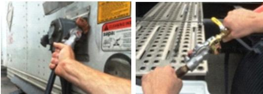
Connect the INJECT-AIR's entry glad hand to the tractor's trailer air supply line (red).
