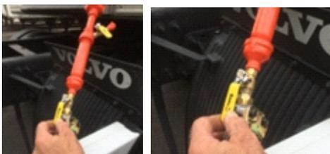
Slowly open the INJECT-AIR's air control valve and charge air system for approximately 2 minutes then close the control valve.
