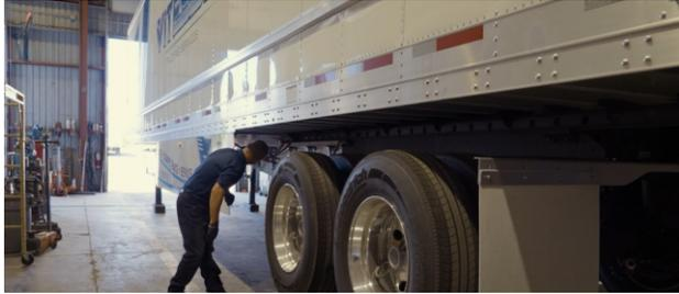
After treatment, walk around trailer for inspection. If it's leaking you will see white bubbles from piping. Close main valve, drain the tanks.
