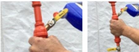
Incorporate 50 mL ALD-3 treatment fluid in the INJECT-AIR's fluid reserve and shut the reserve valve. See page 2 for recommended dosage.
